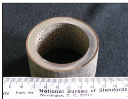
Fig. 3 — A section of the final bimetallic tube produced after coextrusion. The tube has an outside diameter of 2.5 in. with a 0.250-in. wall thickness and a coating thickness of 0.085 in. The final tube length was approximately 20 ft.
